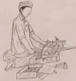
A HALF SELF MADE LATHE IS USED TO APPLY LAC TO WOOD
